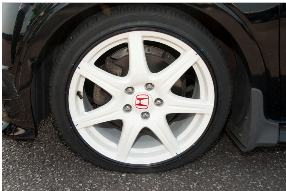
Figure 3 – 'Tyre 2' after at Testing at 0.8 Bar
