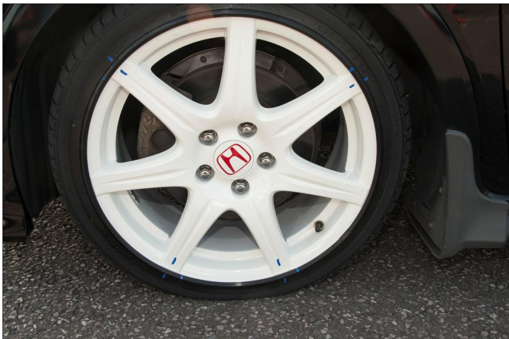
Figure 5 – 'Tyre 3' after Testing at 0.8 Bar
