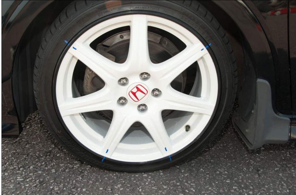
Figure 4 – 'Tyre 3' after Testing at 1.0 Bar
