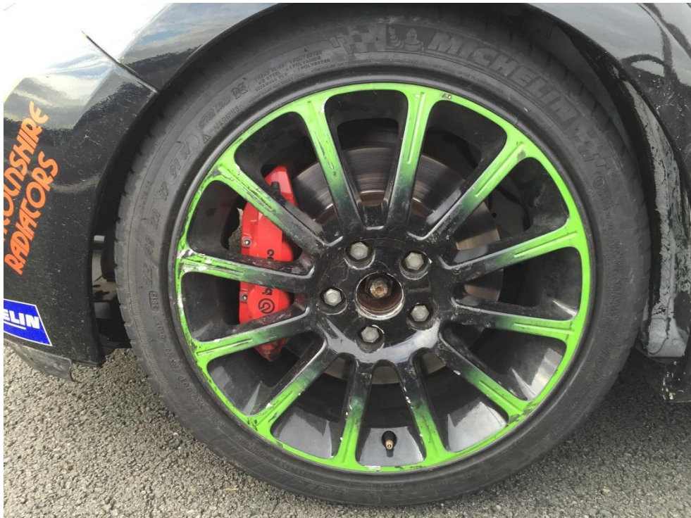
Figure 8 - Wheel, tyre and AlloyGator OE assembly, post Cornering Test
