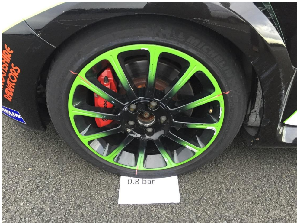
Figure 1 – Standard wheel and tyre assembly, post Tyre Rim Roll-off Test
