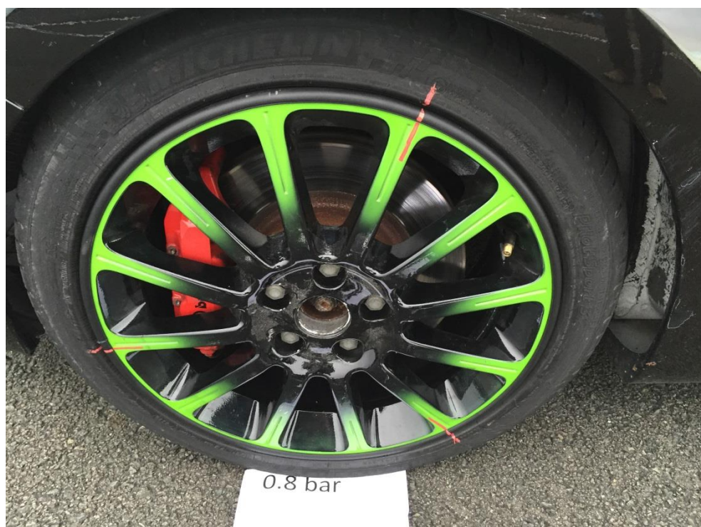
Figure 2 – Wheel, tyre and AlloyGator OE assembly, post Tyre Rim Roll-off Test
