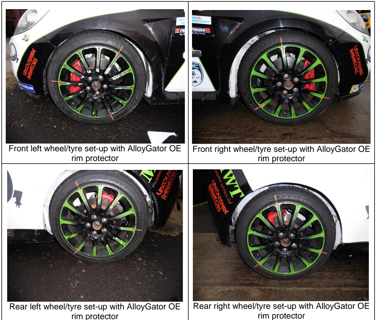
Figure 1 - Wheel/Tyre Set-ups with AlloyGator Rim Protectors
