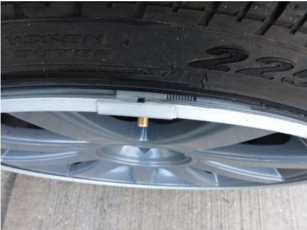
Figure 5: Total movement to the AlloyGator on the LHS rear wheel following completion of Tests 4 and 5
