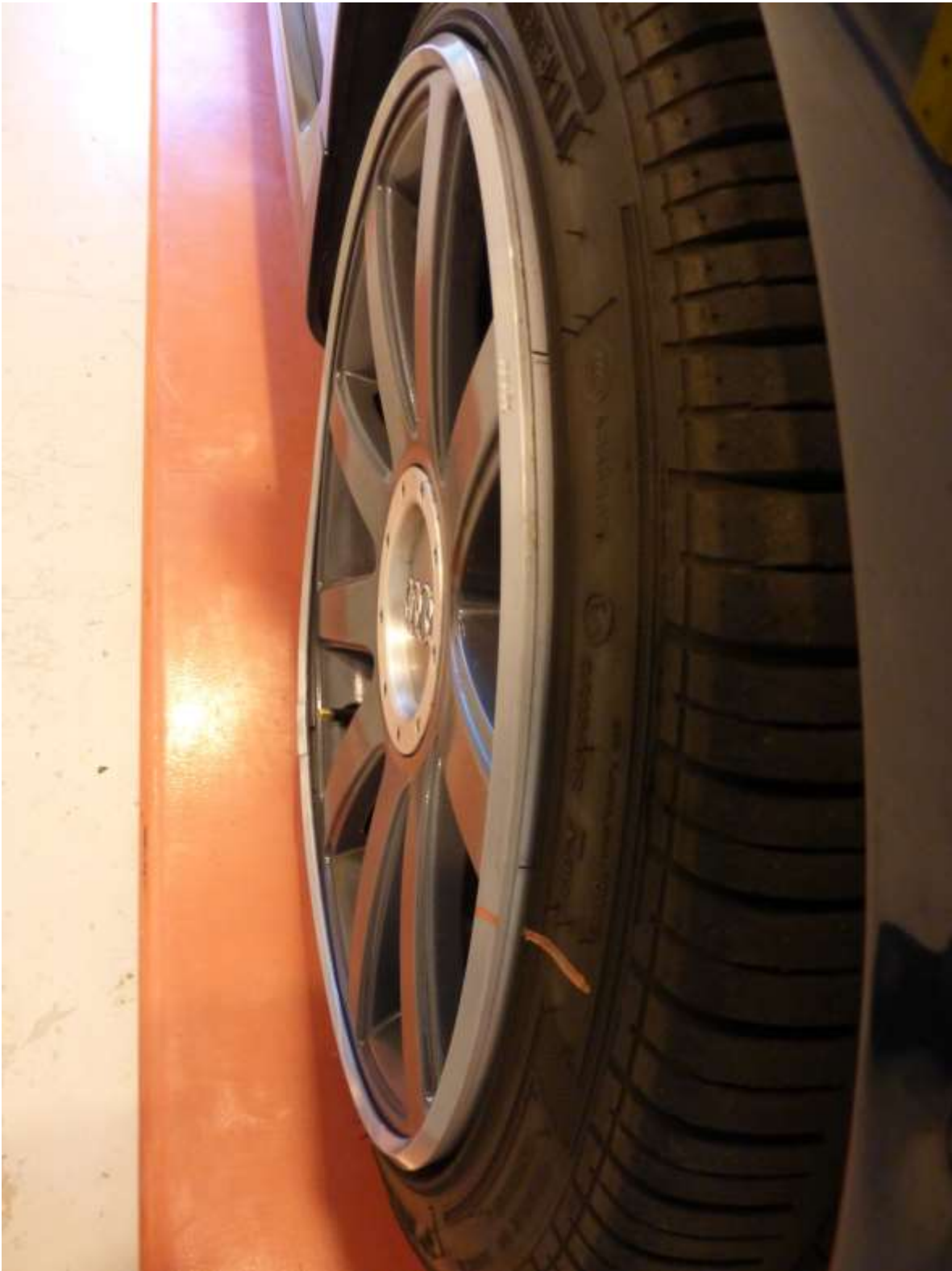
Figure 3: Movement to the AlloyGator rim protector on the RHS front wheel following completion of Test 2
