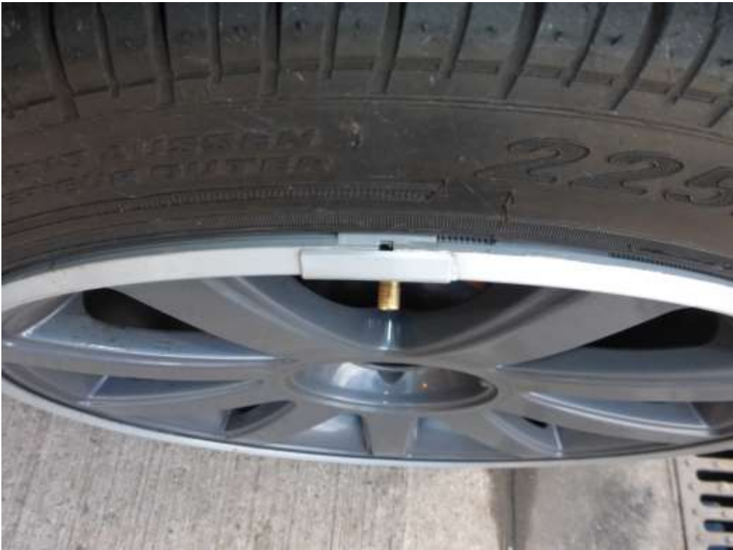
Figure 4: Movement to the AlloyGator on the LHS rear wheel following completion of Test 4
