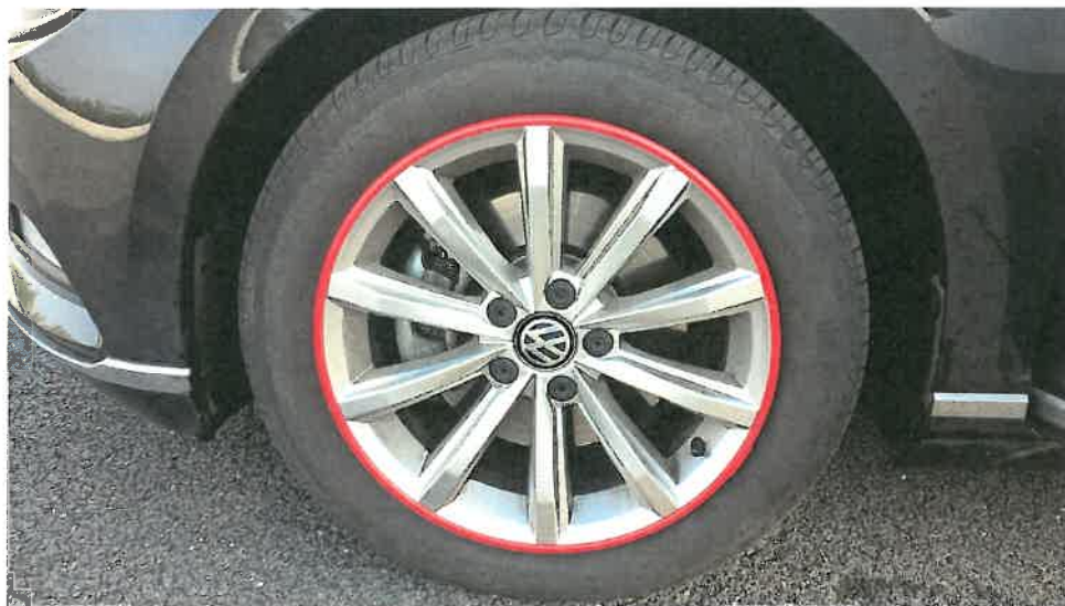
F3 Wheel disc with protection ring AG24 Position of protection ring before tire pressure measurement
