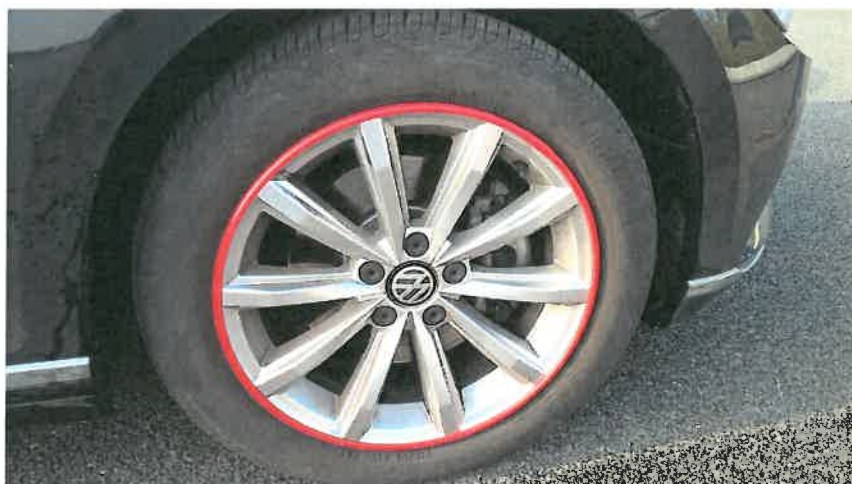
F1 Wheel disc with protection ring AG24 Position of protection ring before test
