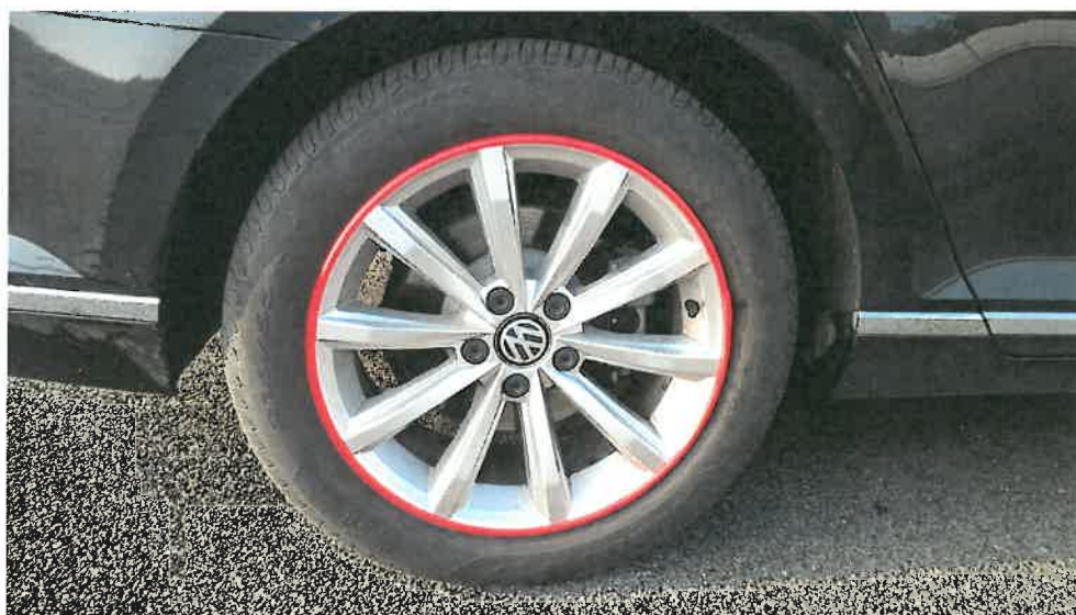
F2 Wheel disc with protection ring AG24 Position of protection ring after driving test
